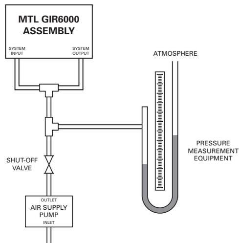
**Figure 7.3** - Leak test apparatus
