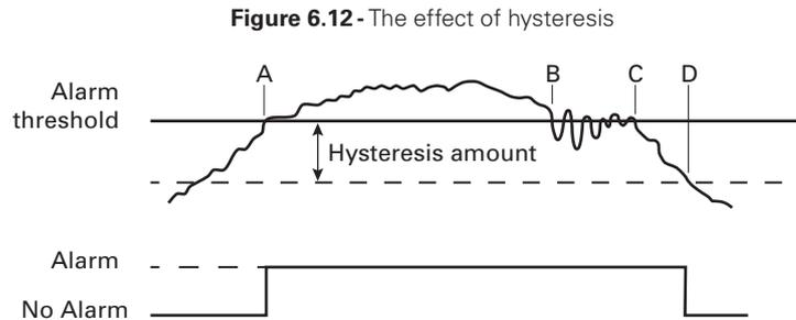
With hysteresis, the level must fall well below the alarm threshold by an amount defined with the hysteresis parameter before the alarm state is 'cancelled' (point 'D').
