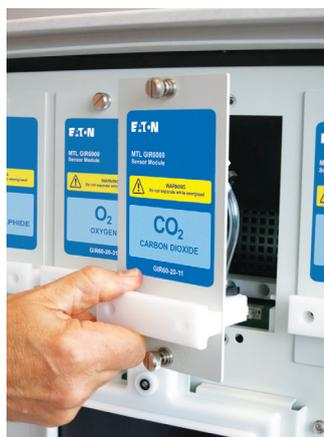
Figure 7.1 - Module removal
