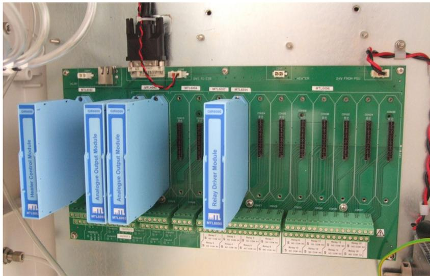
**Figure 4.2-** Signal processing motherboard showing connection terminals
