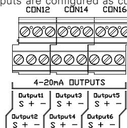
work into load resistances of up to 700 ohms. A terminal is also provided for the cable shield wire.
