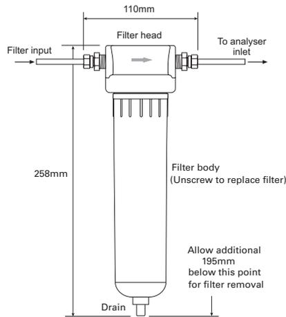
**Figure 3.5** - Standard (optional) coalescing filter on gas inlet
