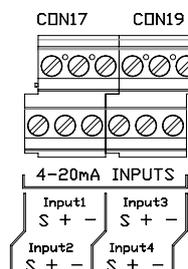
panel. They operate over the conventional current loop 4-20mA range – driving into the '+' terminal and returning via the '-' terminal. A terminal is also provided for the cable shield wire.
