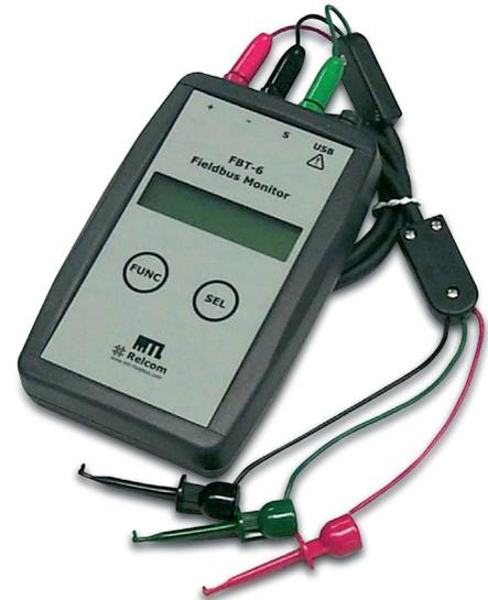
**The Fieldbus diagnostic monitor, FBT-6,** is used to examine the operation of a live FOUNDATION™ fieldbus H1 network without interfering with its operation. The Monitor is intended for maintenance personnel to verify network operation or to troubleshoot an errant network.
