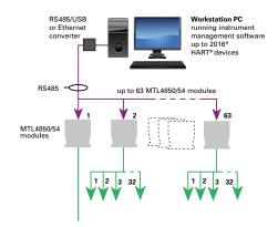
The module has a compact self-contained structure which enables optimised and repeatable performance due to fixed capacity, 32 channels, per module. The unit is ideally suited to enhance existing and new installations.
