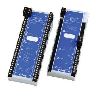
MTL830C analog multiplexer system with Modbus<sup>®</sup> outputs provide a cost-effective alternative to single-loop isolation. The cost of installed wiring is reduced by up to 50% by communicating the input of multiple hazardous-area sensors over a single twisted pair data highway. Further savings are achieved by reducing the number of inputs to the host, cabinet space and weight.
