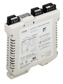
The F101 and F102 fieldbus power supplies are designed to provide power for a single FOUNDATION<sup>TM</sup> fieldbus H1 segment. Galvanic isolation, power conditioning and segment termination are incorporated into each F101 or F102 module. Termination of the fieldbus segments is normally enabled with a switch on the module, but may be switched off for those few applications that do not require a Terminator at the Fieldbus Power Supply.
