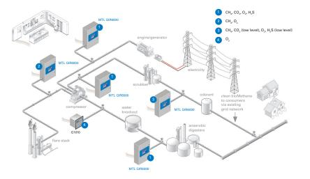
We specialise in the manufacture of hazardous area (ATEX) certified MTL Biogas analysers, wireless communications and surge protection equipment for anaerobic digester (AD) plant installations.
