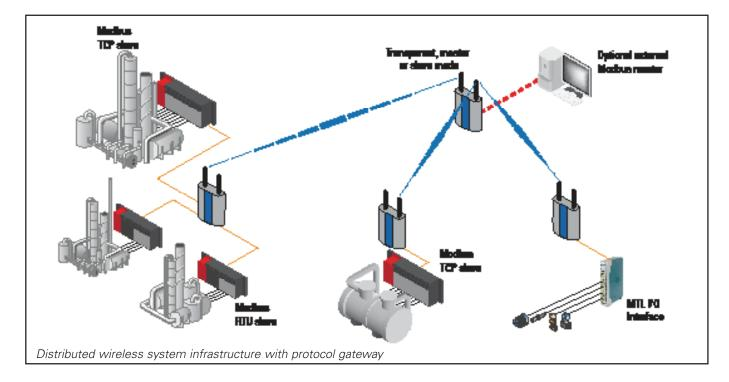
The diagram above represents an installation in which the radios not only communicate between each other, but also convert from one protocol to another. This example is based on a subset of a small, remotely monitored, pumping station.
