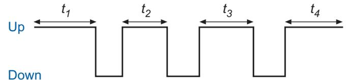
From this we can see what is meant by Up Time – the time when the equipment is available – and Down Time – the time when the equipment has failed and so is unavailable.
