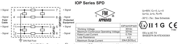
CAUTION: For use in an environment, IOP must be mounted in a suitable enclosure.
