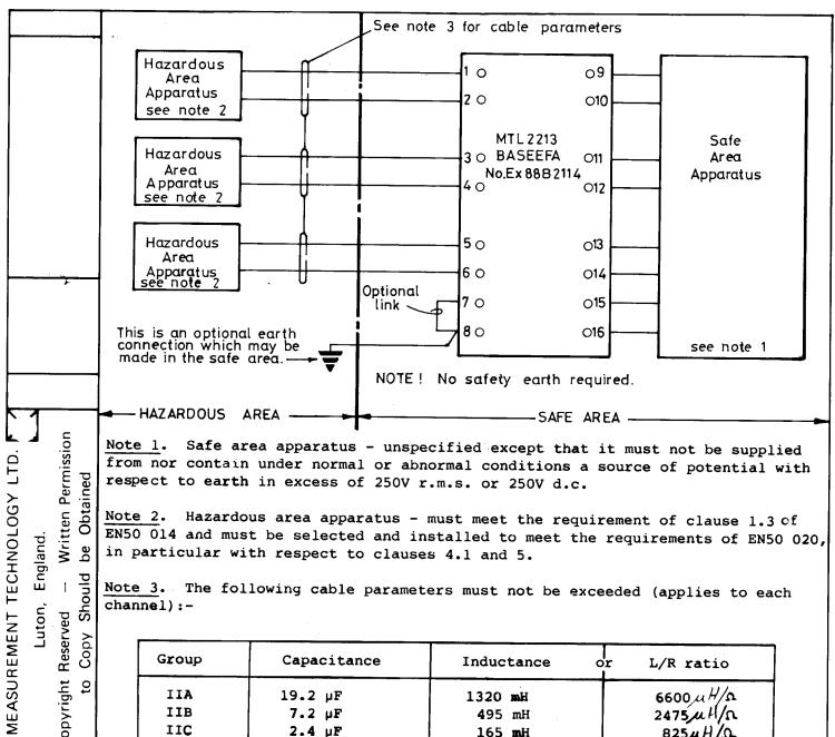
Note 2. Hazardous area apparatus - must meet the requirement of clause 1.3 of EN50 014 and must be selected and installed to meet the requirements of EN50 020, in particular with respect to clauses 4.1 and 5.
