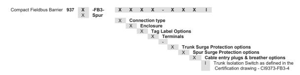
The "X"s represent character positions that can be Alpha-numeric (0-9 or A -Z) and the resulting 18 character part number will result in a design specific code where all features are covered and permitted within drawing – CI9373-FB3-4, and also covered by this certificate
