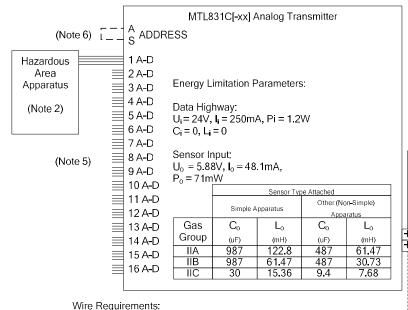
Data Highway Plug Terminals: 0.2 - 2.5 mm<sup>2</sup> (12 - 24 AWG) Input Channel and Address Terminals: 0.14 - 1.5 mm<sup>2</sup> (16 - 26 AWG)
