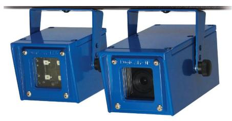
window bezel that fixes to the main housing using hex screws and with an O-ring to provide ingress protection. The electronics are partly encapsulated and fitted inside the housing with a lid using hex socket head screws and with an O-ring to provide ingress protection.
