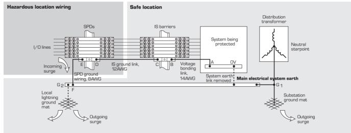
Figure 4 Recommended earthing system for loops including IS barriers and SPDs
