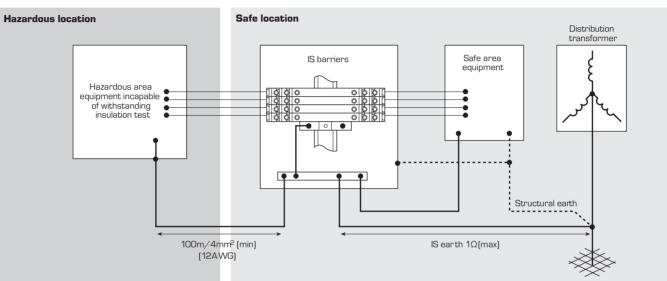
Figure 5 Potential equalizing conductors - UK practice
