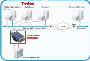
For example, as illustrated in the figure shown here, a 2-port serial device server shares its ports with 4 different hosts.
