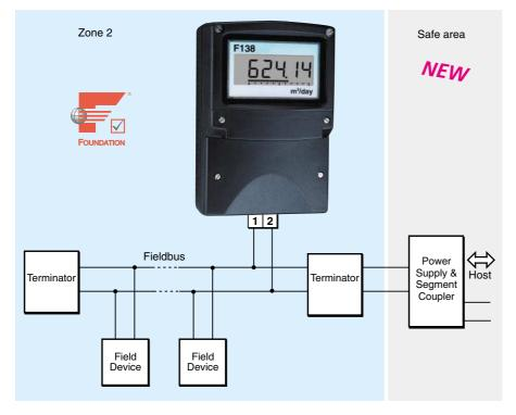
The BA414NDF Fieldbus Display is a new cost-effective Type nL field mounting instrument that can display a single fieldbus process variables in a Zone 2 or Zone 22 hazardous area. Housed in a robust IP66 GRP enclosure, the instrument has a large, high contrast five digit display, plus a horizontal bargraph. The BA414NDF uses the same technology and compliments the well established BEKA eight variable fieldbus displays that are now in worldwide use.
