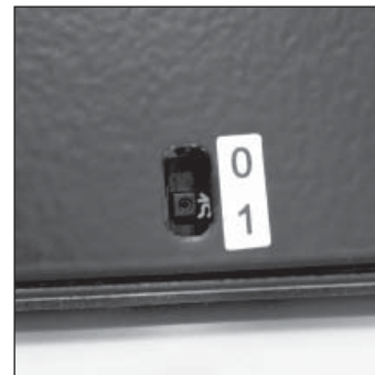
Figure 2-7: Ground reference switch set to '1'
