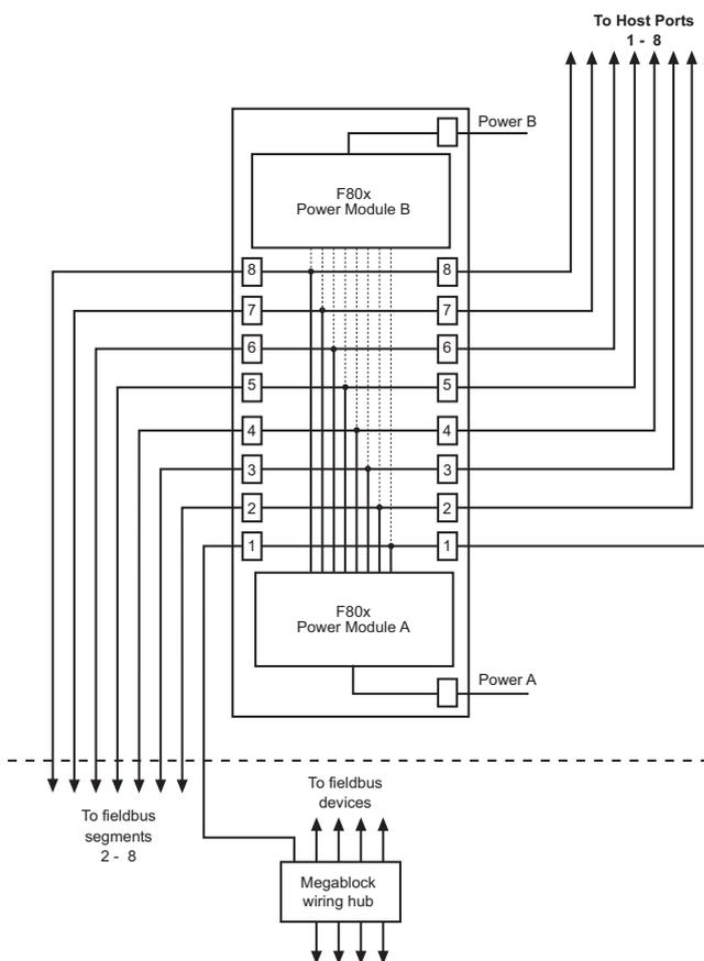
The above diagram shows a block diagram of how the F890 is wired. Note that the Chassis Ground and Alarm connection are not shown. The Diagnostic module is also not shown (see the F809F product specification). For detailed wiring information see the Installation Instructions for the F890 (Document number 502-090).
