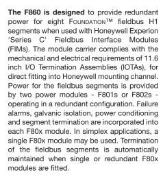
**For extreme reliability**, the F860 IOTA is passive and only provides interconnections between the power modules and the external connections.
