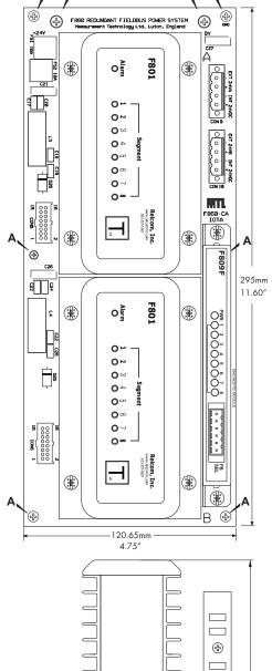
Shown using F801 power modules. Overall dimensions are the same when F802 modules are fitted.
