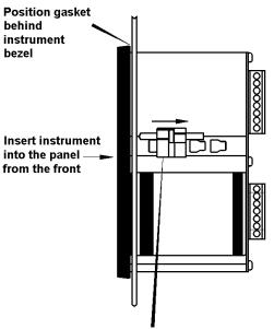
Slide panel mounting clip into the slotted rail on the side of the enclosure. Four clips are required to achieve an IP65 seal between instrument and panel.
