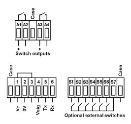
Fig 7 Installation and terminal connections
