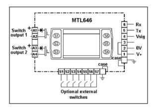
Fig 1 Simplified block diagram of MTL646
