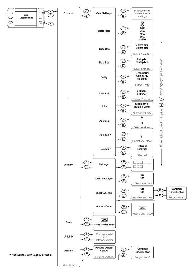
Fig 8 Structure of Configuration Menu
