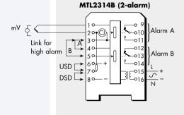
All contacts shown in alarm condition (relay de-energised)
