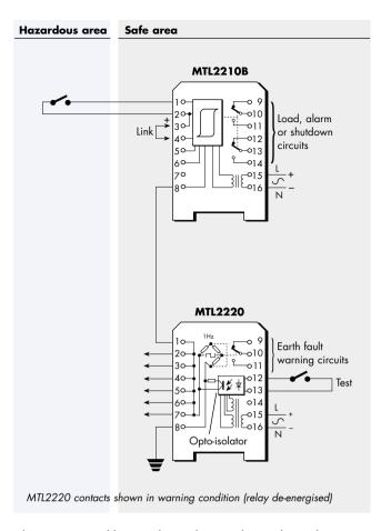
Please note, in addition to the application shown above, the MTL2220 can also be used with most analogue signals.
