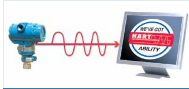
The HART protocol allows additional information to be carried on the same pair of wires with the 4-20mA analogue signal. Simultaneously and Transparently
