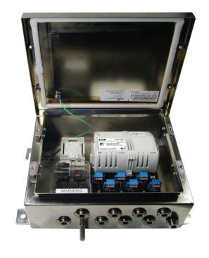
The key modular components of the system (Fieldbus Barriers and Surge Protectors) may be 'hot-plugged' by design and without gas-clearance procedures or separate isolating switches. This virtually eliminates the risk associated with hazardous area maintenance activities, speeds module replacement and avoids the need for specialist operator training.
