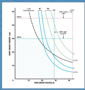
Intrinsic safety is fundamentally a low energy technique and consequently the voltage, current and power available is restricted. Figure 1.1 is a simplified illustration of the available power in intrinsically safe circuits and attempts to demonstrate the type of electrical installation in which the intrinsically safe technique is applicable.
