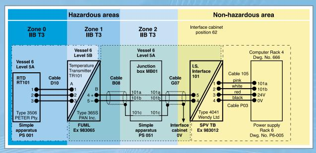
Figure 3.1 - Typical installation drawing for IS system
