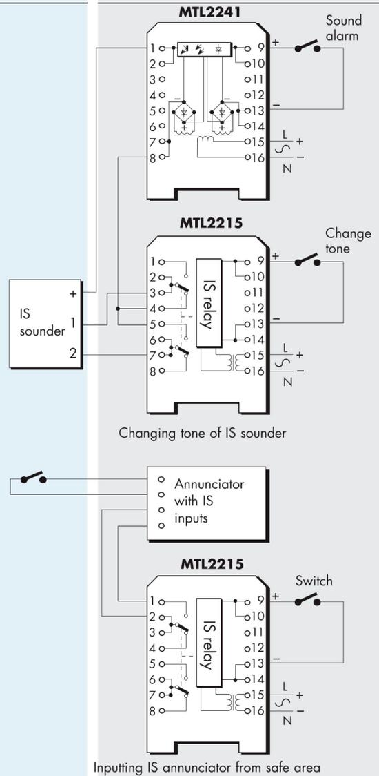
All contacts shown in alarm condition (relay de-energised)
